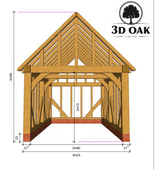
To be mounted on 0m230 plinth. Section sizes provided on request
